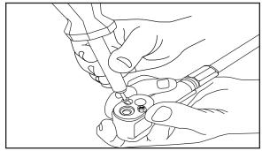
3. Remove old seals and install new seals in the same orientation.
