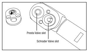
4. Reinstall the face plate, noting its orientation. The smaller hole on the face plate goes over the smaller hole on the seal. Tighten the face plate bolts to 10-15 in-lbs.
