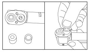
2.Note orientation of seals in the pump head.
