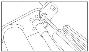
3. Wrap threads of new hose with PTFE tape 2 to 3 full turns.
