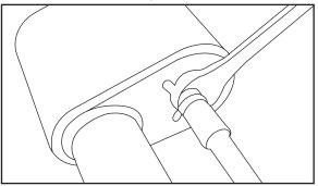
4. Install new hose into pump. Since the threads are tapered pipe fittings, you can thread in by hand until hand-tight. Then, using the 9/16" wrench, tighten an additional 2-3 full turns. If equipped, reinstall hose clip.
